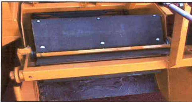
RUBBER PADDLE WHEEL ASSISTS GARLIC ONTO CONVEYER CHAIN.
