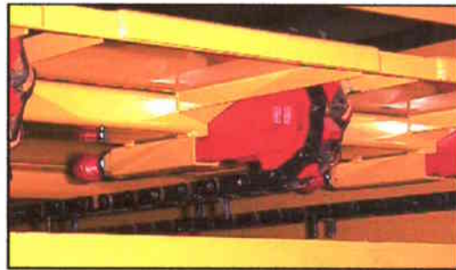
Three individual chain take-up sprockets are steel with 1" sealed ball bearings. The take-up brackets are constructed of heavy steel and 1" take-up bolts. Years of experience have proven it necessary to make this unit very sturdy to withstand the stress of reversing the chain.
