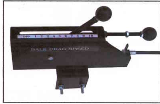
Bale drag speed is controlled from the cab by this cable operated remote control.
