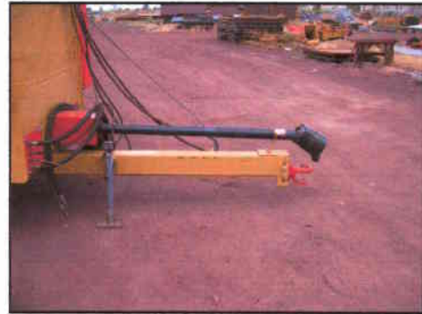
All main drive shafts are made of 1-3/4" alloy material. The over running clutch and slip clutch on the main drive shaft are covered by a hinged safety shield for easy access when servicing. A swing up mechanical screw jack is used for easy hook-up. Also comes with a constant velocity (cv) joint for more angle maneuverability and smooth operation.
