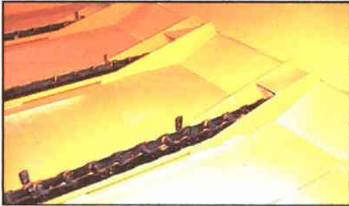
Hay stripper helps to prevent loss of hay. The bale drag chains enter a slotted incline to lift baled hay away from the risers and prevents hay from being pulled down around the sprockets and dropping to the ground, which can waste a lot of hay over time.
