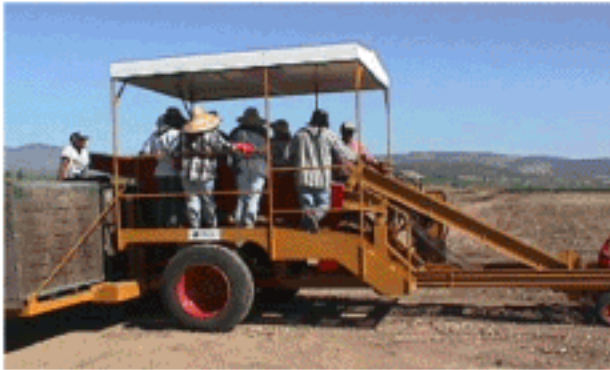
ALL WHITE PAINTED STEEL CANOPY FOR COOLNESS AND COMFORT FOR WORKERS.
