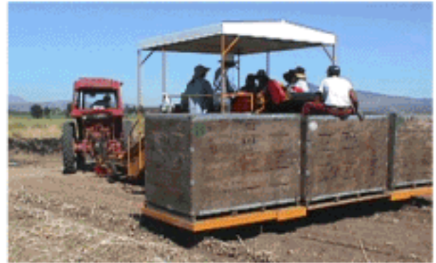
THIS REAR VIEW SHOWS THREE TOTE BOXES, THE OUTER TWO ARE THE EMPTIES. CENTER PLATFORM WILL LOWER FULL BOX TO THE GROUND WHEN FULL.
