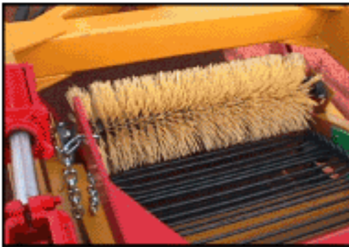
ADJUSTABLE SPEED ROLLER STYLE BRUSH GENTLY ASSIST GARLIC ON TO THE ELEVATOR.
