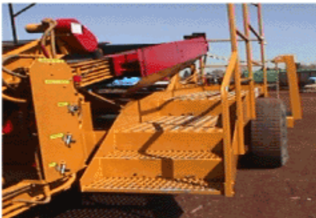
NO SLIP CAT WALKS AND STEPS WITH SAFETY RAILS.
