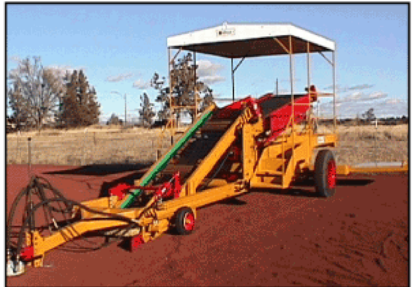
THIS FRONT VIEW SHOWS LARGE HYDRAULIC PUMP HOSES WHICH ARE SUSPENDED BY A SPRING LOADED POGO STICK. ALSO SHOWN IS AN ADJUSTABLE CATEGORY 3 HITCH.
