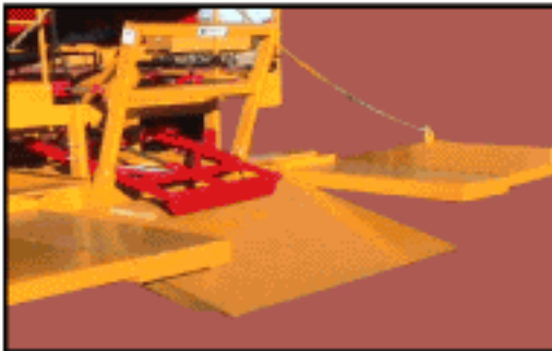
A CLOSE-UP VIEW OF THE HINGED PLATFORM AND PUSH-OFF IN THE UNLOADING POSITION.
