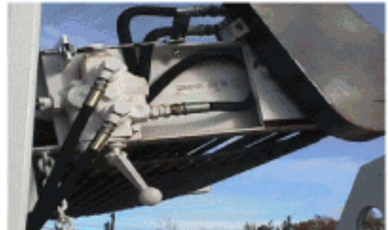
THIS HANDLE CONTROLS THE LOWERING AND RAISING OF THE FILLED BOX PLATFORM AND PUSH-OFF. NOTE! WILL NOT FUNCTION IF CONVEYORS ARE IN MOTION, THUS PREVENTING GARLIC FROM FALLING OFF THE CONVEYOR AND TO THE GROUND.
