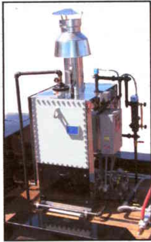
A STEAM BOILER IS REQUIRED FOR OPERATION OF THE NEWHOUSE ESSENTIAL OIL STILL
