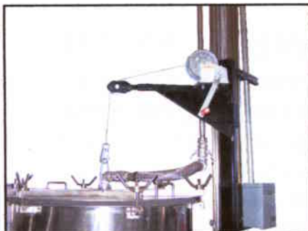
WINCH PROVIDED TO LIFT 3/16" S.S. PLATE COVER
