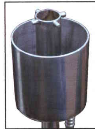
SECONDARY WATER DISCHARGE TO ADJUST HEIGHT OF OIL LEVEL IN GLASS BEAKER
