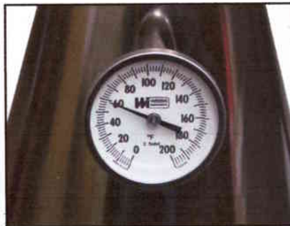
TEMPERATURE GAUGE ON THE TP RECEIVING CAN, FOR PROPER TEMPERATURE
