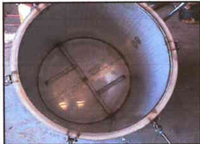
INSIDE VIEW OF THE COOKER POT WITH SCREEN REMOVED TO REVEAL SPECIALLY DESIGNED MANIFOLD, FOR PROPER STEAM DISTRIBUTION
