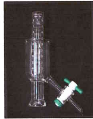
CLOSE UP VIEW OF GLASS BEAKER, SHOWS OIL/WATER LEVEL, OIL OVER FLOWS FROM SEPARATING TUBE INTO OUTER COLLECTION VESSEL THAT HAS A VALVE TO DISCHARGE OIL INTO A COLLECTION CONTAINER
