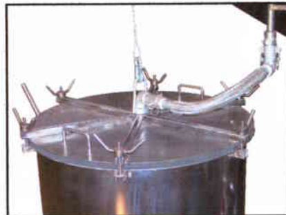
3/16" S.S. PLATE LID IS SECURED DOWN TO THE COOKER POT WITH 6 SCREW DOWN CLAMPS
