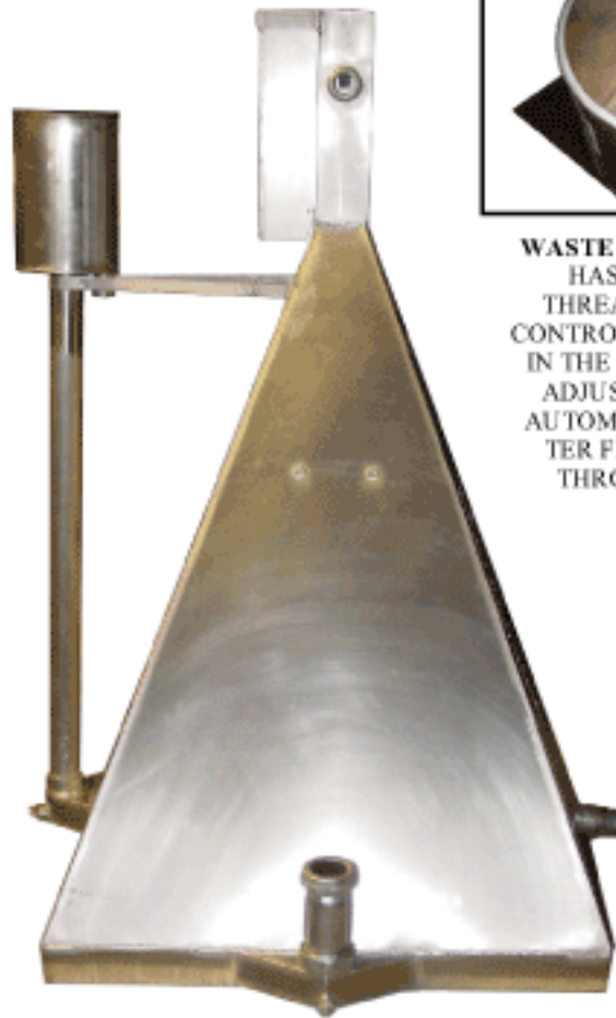
VIEW OF COALESER WITH NEARLY 7,000 sq in OF COLLECTING SURFACE
