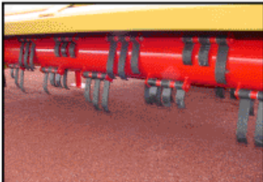
LARGE HEAVY DUTY ROTOR WITH CUPPED FLAILS .
