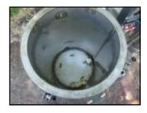
COOKER POT IS MADE FROM STAINLESS STEEL TO ASSURE NO OIL CONTAMINATION AND LONG TROUBLE FREE LIFE
