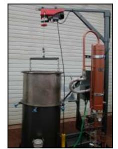
AN ELECTRIC HOIST IS PROVIDED TO LIFT THE STAINLESS MATERIAL BASKET OUT OF THE COOK POT ASSEMBLY AND INTO THE DUMP STAND ASSEMBLY.
