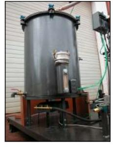
AUTOMATIC WATER LEVEL CONTROL, AUTO PILOT IGNITION, LOW WATER SHUT-OFF AND WATER INLET PRE-HEATER ARE JUST A FEW OF THE HIGH QUALITY FEATURES THAT ARE STANDARD ON THIS NEWHOUSE DISTILLATION
