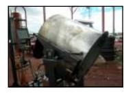
STAINLESS MATERIAL BASKET PLACED INTO THE DUMP STAND ASSEMBLY AND IN THE DUMP POSITION
