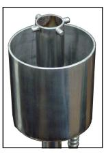
SECONDARY WATER DISCHARGE TO ADJUST HEIGHT OF OIL LEVEL IN GLASS BEAKER
