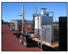
AN ALUMINUM FEED WATER TANK IS INCLUDED TO FEED THE BOILER AND FOR CONDENSER COOLING WATER
