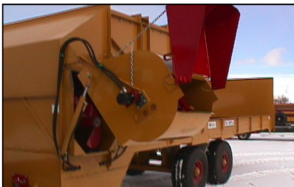
TWIN HYDRAULIC CYLINDERS USED TO RAISE BLOWER AWAY FROM DISCHARGE AUGER IF PLUGGING STARTS
