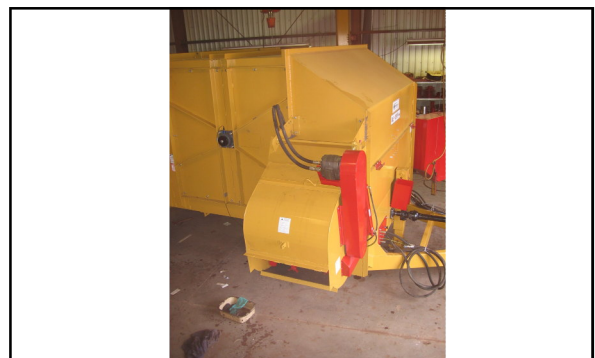
NEW HYD PUMP AND BELT DRIVE INCREASE AIR FLOW
