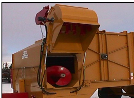
RAISED FULLY TO ALLOW MATERIAL TO DISCHARGE WITHOUT REMOVING THE BLOWER. USED FOR BUNKER FEEDING OR DISCHARGING MATERIAL ON THE GROUND
