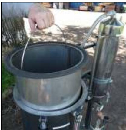
THE REMOVABLE LINER IS FOOD GRADE STAINLESS WITH A SPECIAL DOUBLE SEAL GASKET AND A PERFORATED BOTTOM, THIS ALLOWS EVEN STEAM DISTRIBUTION THROUGHOUT THE MATERIAL
