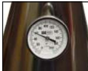
TEMPERATURE GAUGE ON THE SEPARATING CAN, FOR PROPER TEMPERATURE CONTROL OF CONDENSATE
