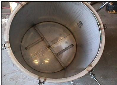
**INSIDE VIEW OF THE COOKER POT WITH SCREEN REMOVED TO REVEAL SPECIALLY DESIGNED MANIFOLD, FOR PROPER STEAM DISTRIBUTION**
