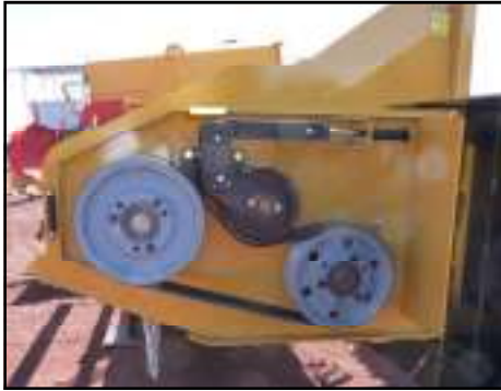
BELT DRIVEN POWER TRAIN 5VX COGGED BELTS, THESE BELTS HAVE A HIGHER HP RATING THAN THE OLD "C" SECTION BELTS.
