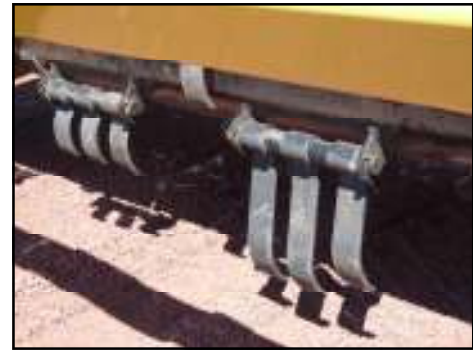
Cupped Knife - The vacuum created by the standard 5/16" thick X 2" wide cupped knives lifts the flattened material into the rotor for a complete and uniform cut.
