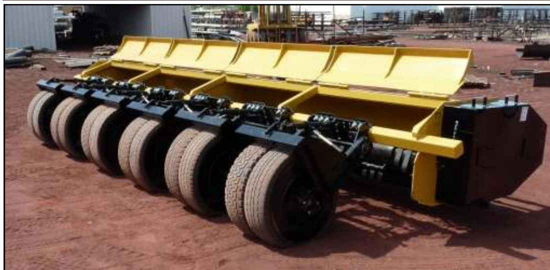
REAR VIEW SHOWING ACCESS DOORS OPEN AND OPTIONAL INDIVIDUAL TIRE ROLLERS
