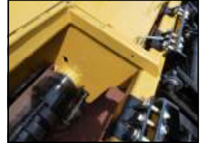
Center drum bearings are QM / Timken heavy duty dual spherical bearings
