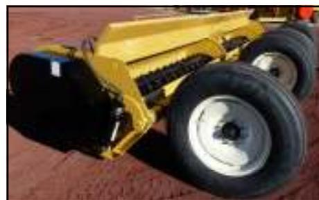
Rear doors have been added to the back. This allows you to run with the doors closed for a very fine chop or open for a high volume coarser broadcast chop. This picture shows the third position which is fully open, this allows for unprecedented access to the drums and bearings for easy maintenance and flail replacement!
